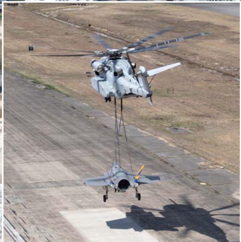
Marine Corps pilots from VMX-1 flying a CH-53K helicopter lower a non-flying F-35C airframe from the NAS Patuxent River F-35 Integrated Test Force onto the runway at Joint Base McGuire-Dix-Lakehurst, New Jersey, April, 24, after transporting the F-35C airframe from NAS Patuxent River, Maryland. The transportation of the airframe will enable future testing at Lakehurst of emergency recovery systems.
