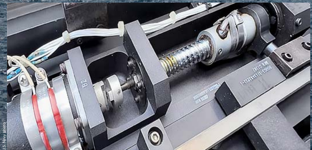
The coupler located inside the Optical Landing System motor assembly.
