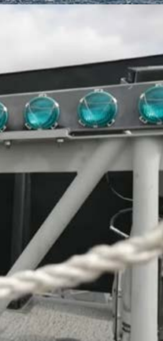
An example of the Optical Landing System like the one aboard the USS Bataan (LHD 5).
