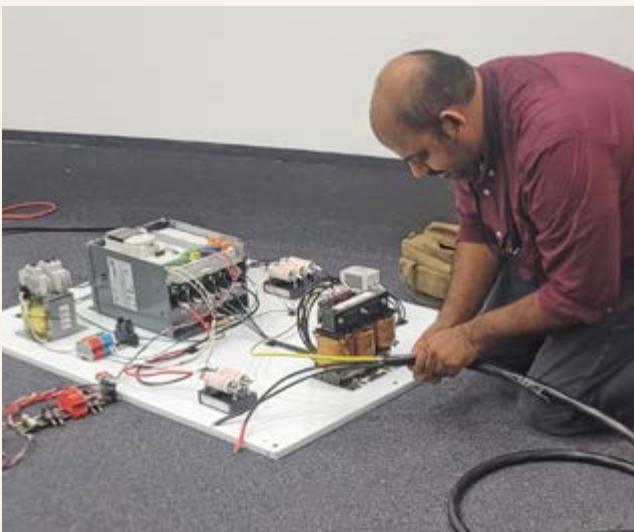
Anil Thomas, a mechanical engineer with NAWCTSD who designed the motor control unit, pictured center, works on the prototype motor control unit for the Multi-Station Disorientation Demonstrator, or the “spin and puke” trainer. Pictured at right is a spare motor from the unit.
