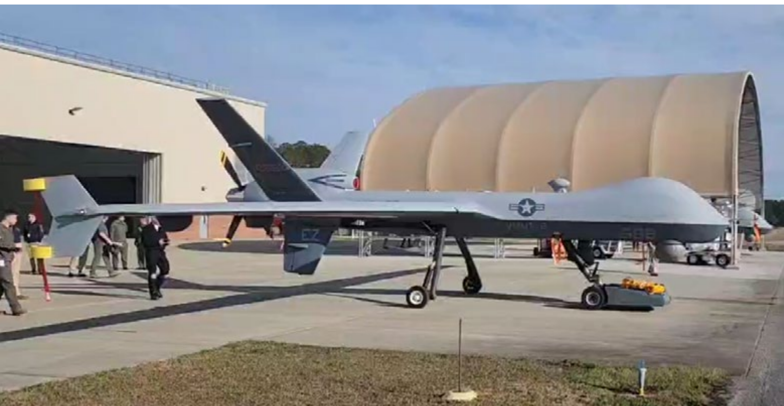
TowFLEXX allows a single operator to maneuver military aircraft with unprecedented precision, maintaining the aircraft's nose wheel alignment while enabling 360-degree turns in confined spaces.
