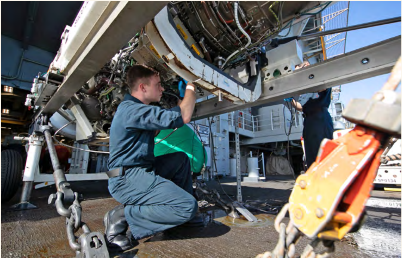
Aviation Machinist’s Mate Airman Joseph Davis assigned to the world’s largest aircraft carrier USS Gerald R. Ford’s (CVN 78) aircraft intermediate maintenance department (AIMD), prepares an F/A-18 Super Hornet engine to be transported into Gerald R. Ford’s engine bay, June 14, 2023.
