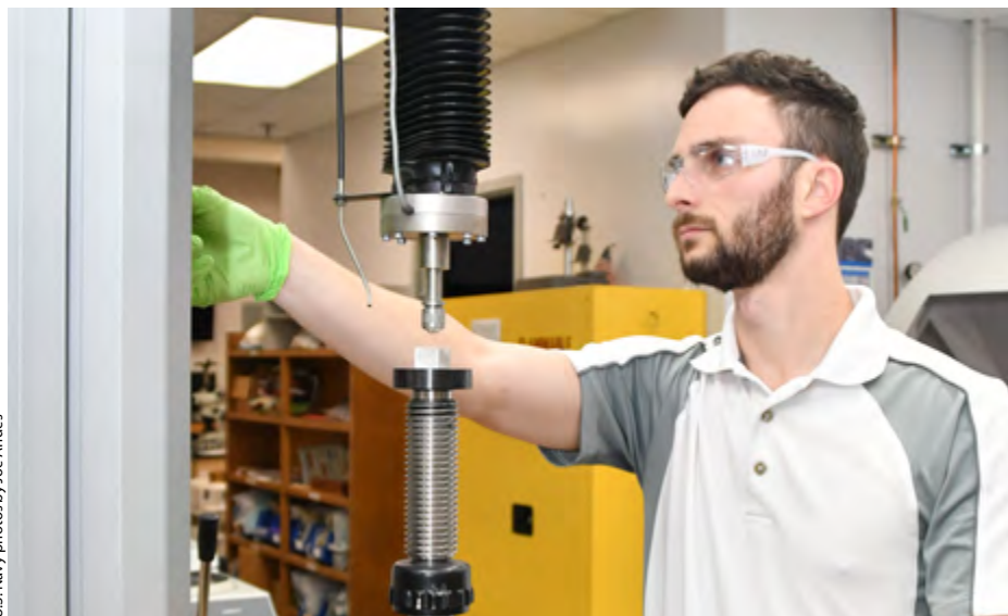
Latane Mason, a materials engineer at FRCE Materials Engineering Division, tests a piece of metal using a macro hardness tester.
