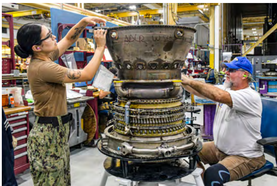
Aviation Machinist’s Mate 3rd Class Natalie Burgos, assigned to FRCSE Detachment Jacksonville, and Aircraft Ordnance System Repairer James Quiett with FRCSE’s engine production team, disassemble an F414 High Pressure Combustion (HPT) Engine Module.
