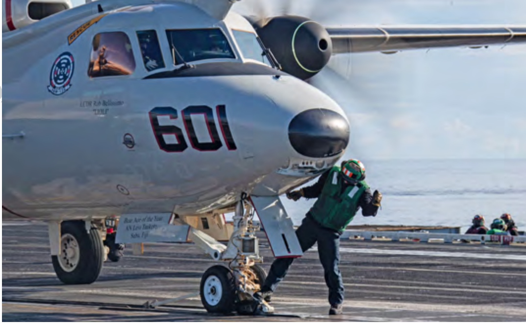
Aviation Boatswain's Mate (Equipment) 2nd Class Hunter Athey, assigned to the air department of the world's largest aircraft carrier USS Gerald R. Ford (CVN 78), sets tension on an E-2D Hawkeye, attached to the "Bear Aces" of Airborne Command and Control Squadron (VAW) 124, on the flight deck. SPB will be rolled out to all type/model/series aircraft.
