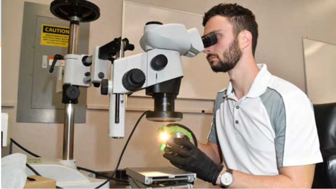
Latane Mason, a materials engineer at FRCE Materials Engineering Division, examines a fractured surface using a stereo microscope.
