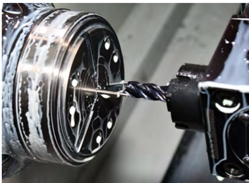
A computerized numerical control lathe at Fleet Readiness Center East (FRCE) manufactures an offset pin for use on an AV-8B Harrier.
