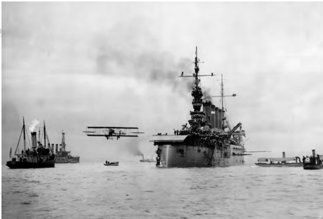
Ely leaves the stern deck of the Pennsylvania just after landing aboard the ship on Jan. 18, 1911. Note the direction of the ship's smoke indicating the crosswind at the time.
