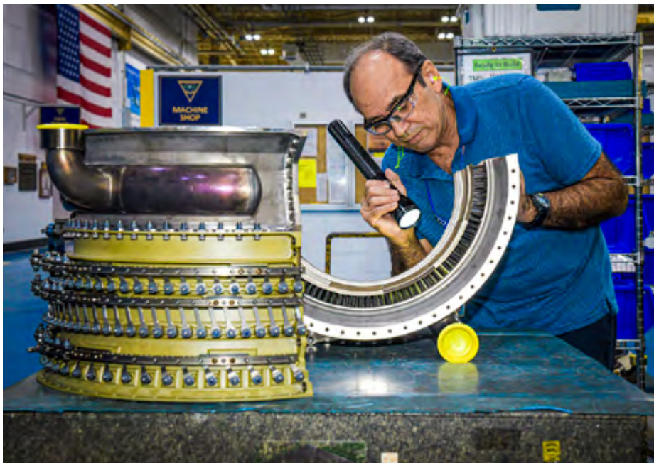
Quality Assurance Specialist Hugo Rodriguez performs a final inspection prior to reassembling an F414 High Pressure Compressor Stator (HPC).
