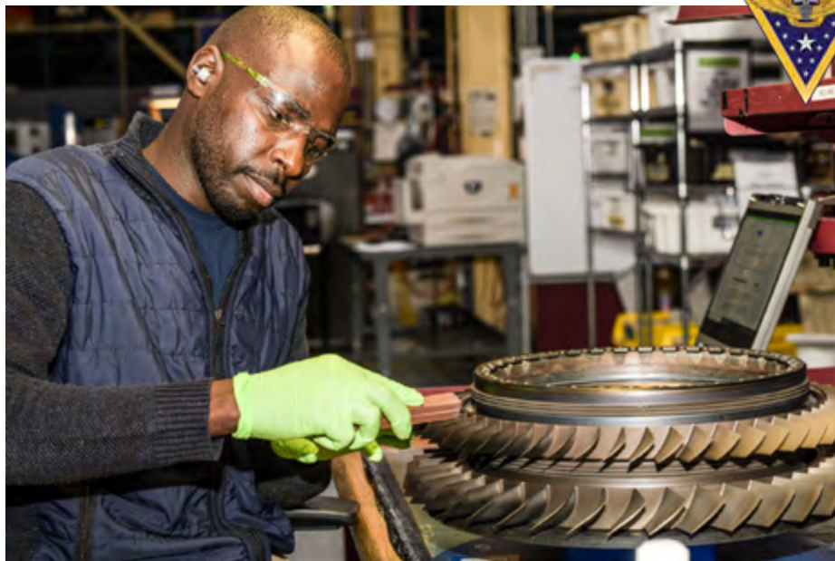
Turbine Power Plant Mechanic Linus Nyamoko blends the first and second stage brisk of an F414 High Pressure Compressor Stator (HPC).
