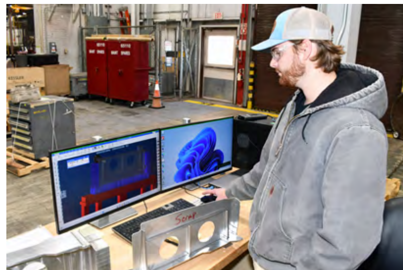
Jack Forehand, a machinist in the Manufacturing Machine Shop at Fleet Readiness Center East (FRCE), scans for potential errors as a rendering of a tool path for an H-53 aft cabin fitting plays through prior to running the part on a five-axis computerized numerical control mill.
