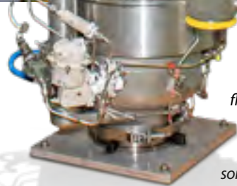
A cross-disciplinary team at Fleet Readiness Center East (FRCE) worked to successfully reestablish capability for the C-2A Greyhound auxiliary power unit (pictured left) when evolving fleet needs resulted in service life extension for the aircraft, which supports the U.S. Navy’s carrier onboard delivery mission. The team included, from left, Justin Rimmer, Engine Driven Compressor and Gas Turbine Compressor Shop supervisor; Edwin Agnes; Erik Dumas, senior engineer with the Naval Air Systems Command Gas Turbine Compressor/Pneumatics Fleet Support Team at FRCE; Anthony Jones; Grady Mayo; aircraft examiner Lawrence Murphy; and production controller Katia Councilman.
