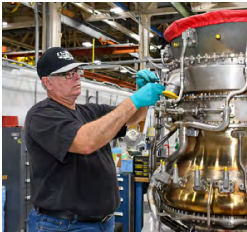
Fleet Readiness Center East (FRCE) engine mechanic Mark Schexnayder begins to disassemble the T408 engine in preparation for maintenance.
