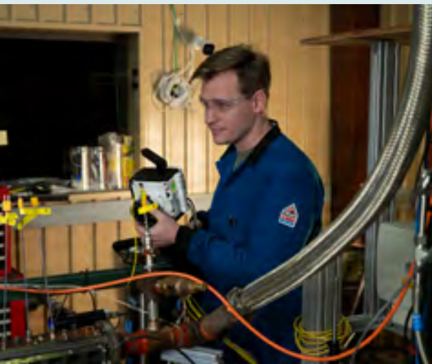
Nicholas Diskerud, Ph.D., Nuclear Regulatory Commission postdoctoral research associate, focuses a high-speed camera on an optically-accessible solid-fuel slab burner at the U.S. Naval Research Laboratory's (NRL) Combustion Lab in Chesapeake Beach, Md., Jan. 15.
