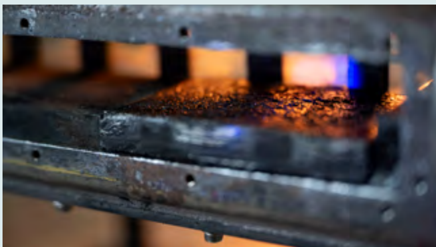
Brian Fisher, Ph.D., U.S. NRL mechanical engineer, adjusts fittings on an optically-accessible solid-fuel slab burner at NRL's Combustion Lab in Chesapeake Beach, Md., Jan. 15.
