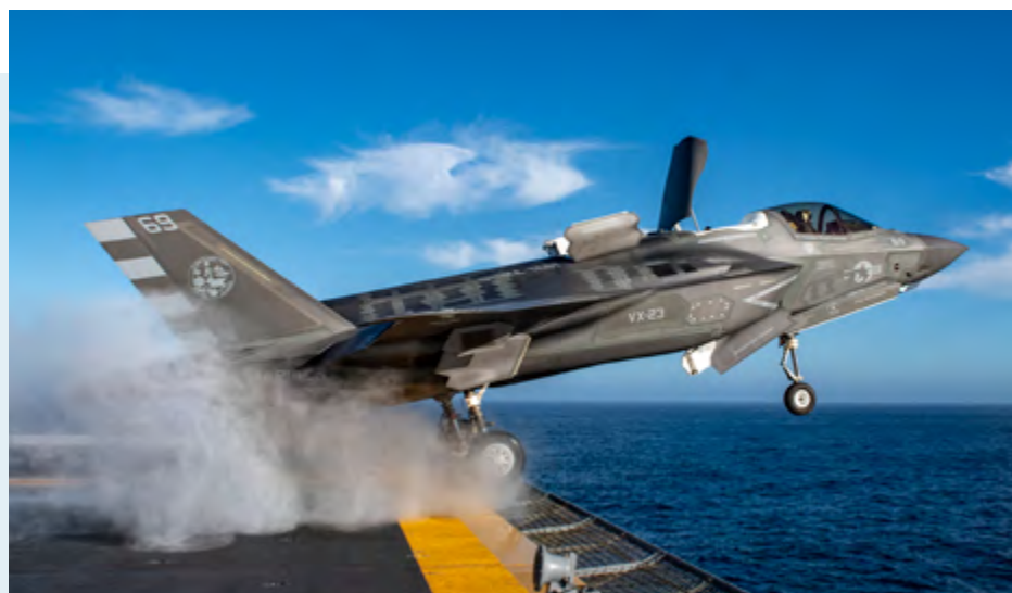
A joint team consisting of F-35 Patuxent River Integrated Test Force flight test members, U.S. Sailors and Marines, and the crew of the Japan Maritime Self-Defense Force Izumo-class multi-functional destroyer JS Kaga (DDH 184), executed developmental sea trials in the eastern Pacific Ocean to gather the necessary data to certify F-35B Lightning II short takeoff and vertical landing aircraft operations.
