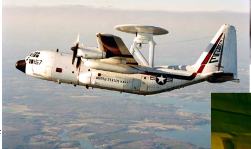
An NC-130H provides an in-flight test bed for a Radar Modernization Program under development for the next generation E-2C “Hawkeye” Carrier Airborne Early Warning aircraft, Oct. 28, 2002.
