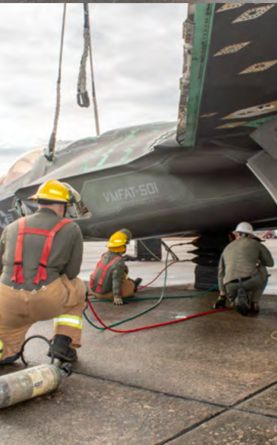
David White, an F-35 support equipment engineer at Fleet Readiness Center East, builds a temporary structure to support the nose of an F-35B Lightning II during aircraft recovery training conducted by Marine Wing Support Squadron (MWSS) 271.
