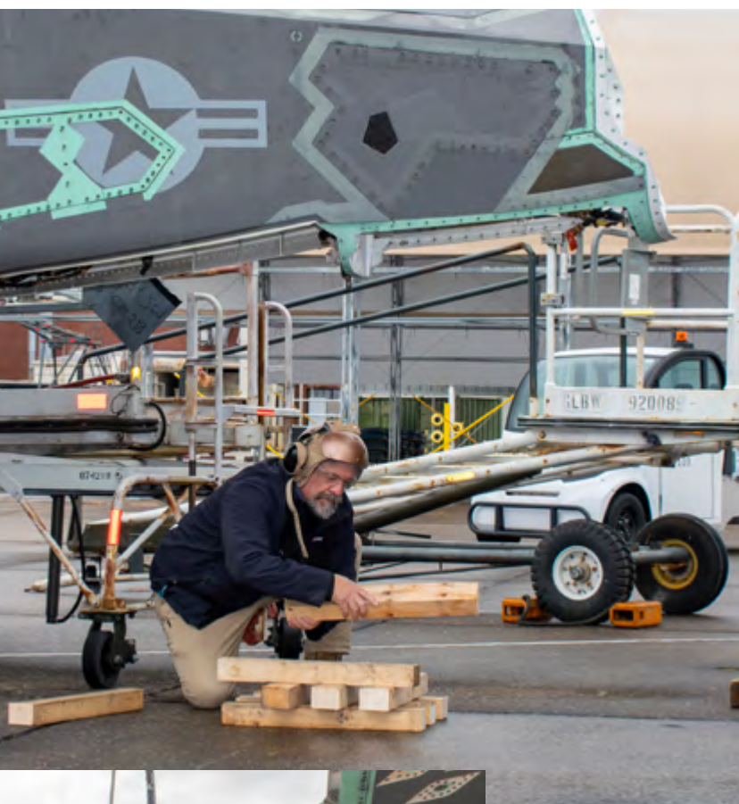
David White, an F-35 support equipment engineer at Fleet Readiness Center East, builds a temporary structure to support the nose of an F-35B Lightning II during aircraft recovery training conducted by Marine Wing Support Squadron (MWSS) 271.
