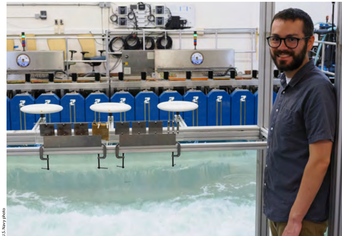
Alex Johnson stands next to symmetric airfoils used to measure the dry deposition of chloride and sulfate. This is used to study the impact of corrosion from saltwater aerosols at the NRL Laboratory for Autonomous Systems Research (LASR) Littoral Bay Wave Pool, in Washington, D.C., Sept. 24, 2024.
