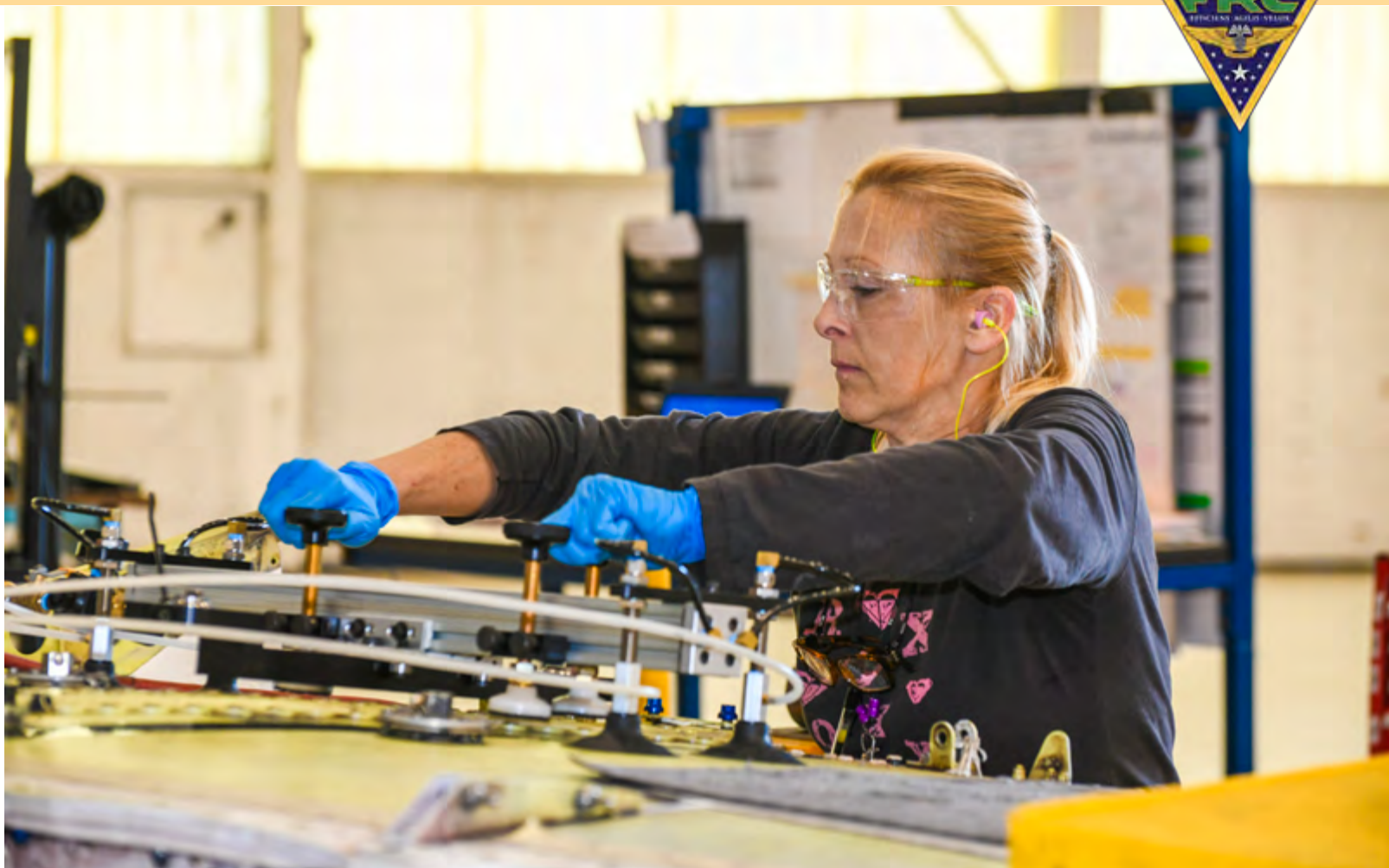
Charlotte Miller, a sheet metal mechanic at Fleet Readiness Center Southeast (FRCSE), prepares to use a drill guide fixture on the center wing section to create precise holes during service life extension program upgrades on a T-45 Goshawk wing, March 27.
