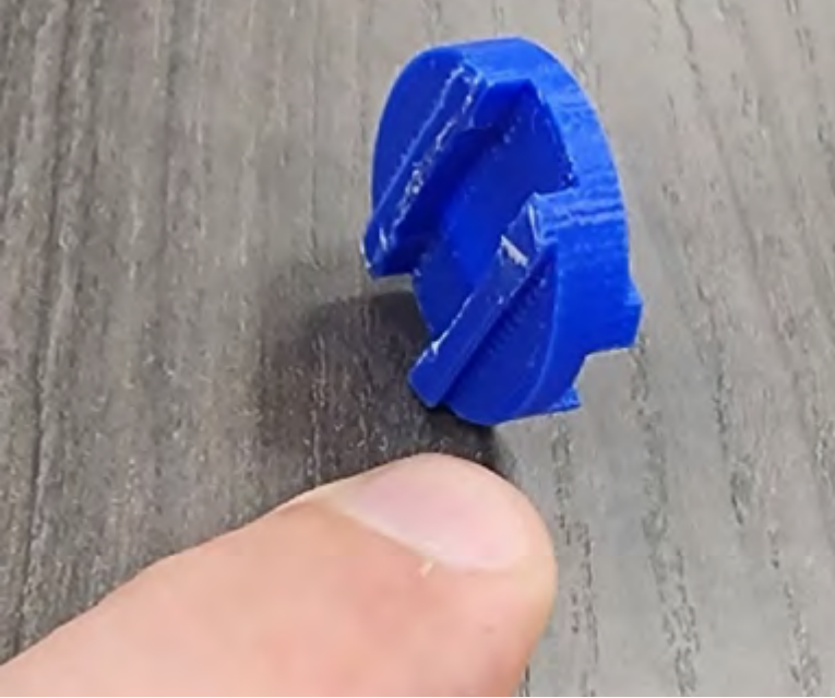
A test coupler printed by the NAVAIR AM team from a similar OLS system the team had addressed a few months earlier than the USS Bataan OLS issue.
