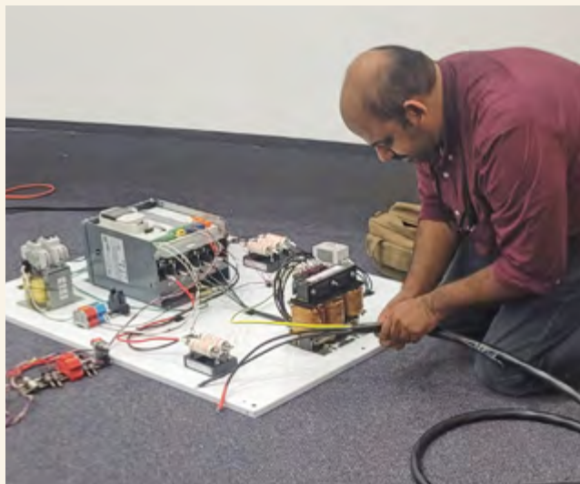
Anil Thomas, a mechanical engineer with NAWCTSD who designed the motor control unit, works on the prototype motor control unit for the Multi-Station Disorientation Demonstrator, or the “spin and puke” trainer. Pictured at right is a spare motor from the unit.
