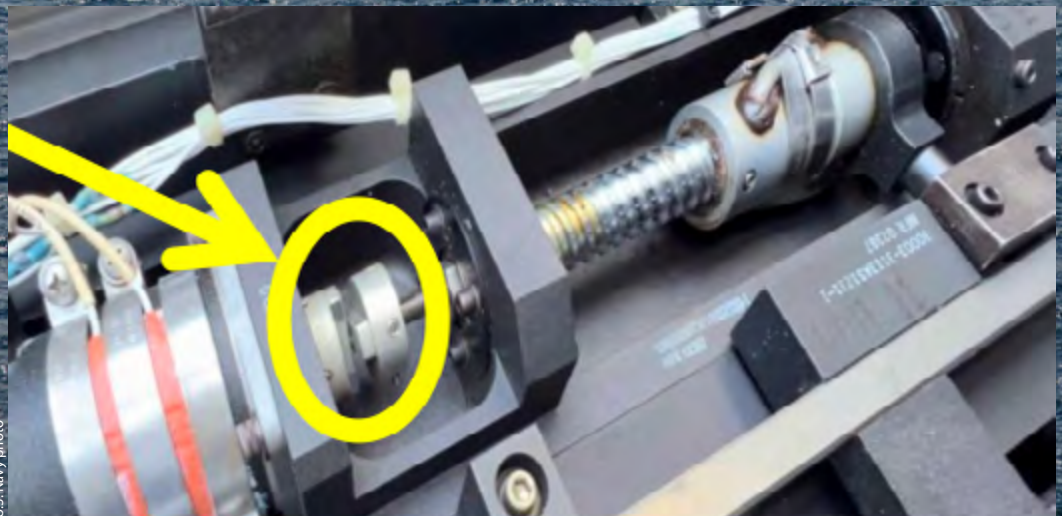
The coupler located inside the Optical Landing System motor assembly.
