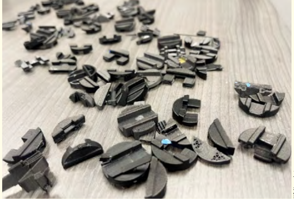
The NAVAIR Additive Manufacturing Team tested more than 20 printed parts for torque strength before arriving at a part that passed the part's unique breakaway requirement.
