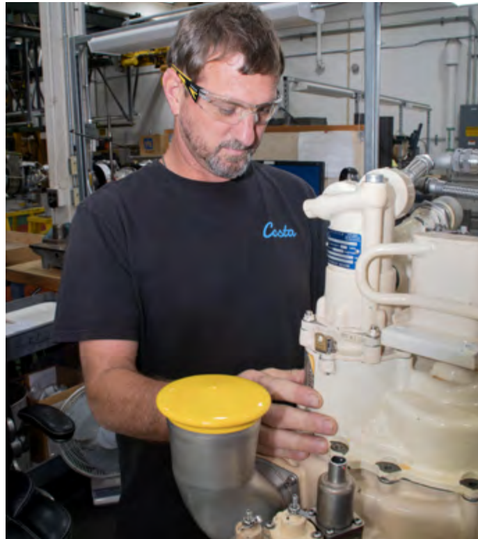
Ryan McNeil, a pneumatics systems mechanic at Fleet Readiness Center East, works on an auxiliary power unit used in the F/A-18E/F Super Hornet.
