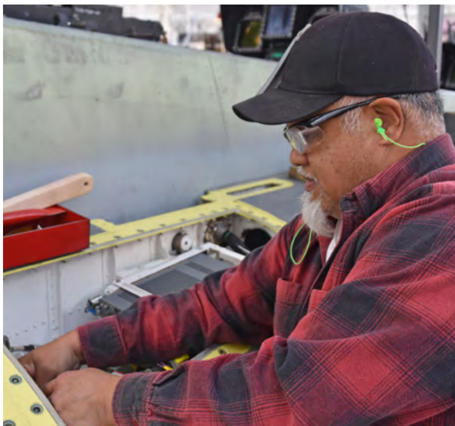
Aircraft electrician Orlando Irwin rewires the leading edge extension wing harness on an F/A-18 Super Hornet at NAS North Island, Coronado, California.
