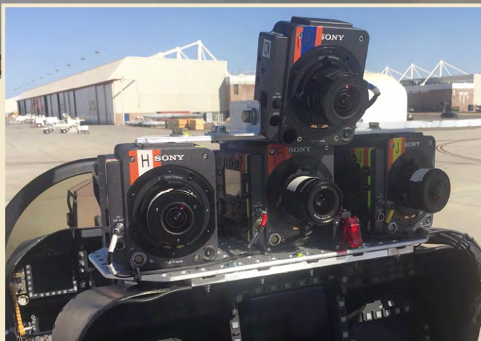
Sony Venice 6K cameras, that weigh about 8 pounds with a lens, were installed on the aft seat's glare shield of an F/A-18.
