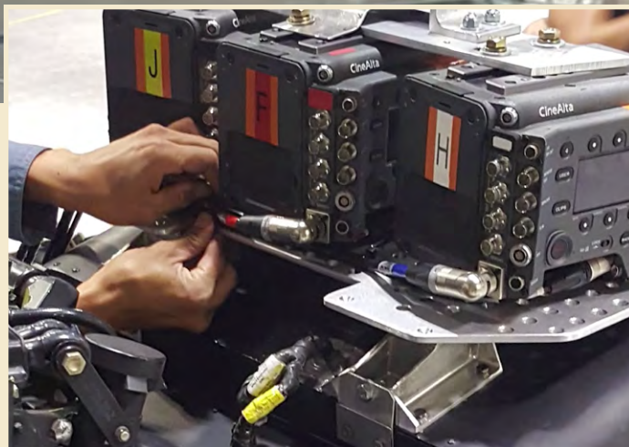
Sony Venice 6K cameras, that weigh about 8 pounds with a lens, were installed on the aft seat's glare shield of an F/A-18.
