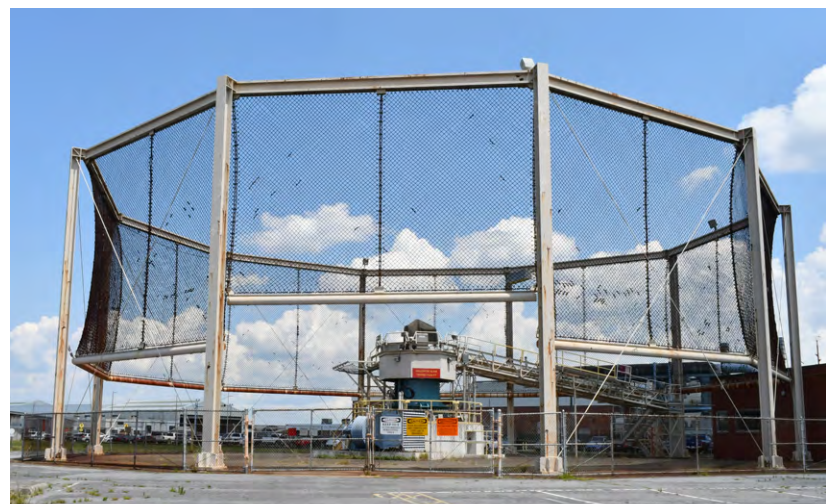
The Helicopter Blade Balance Facility's whirl tower has traditionally been used to balance helicopter rotor blades at Fleet Readiness Center East. However, the H-53K program is opting to use the universal static balance fixture (USBF) instead of the whirl tower to balance its blades, because the USBF can accommodate the increased length and weight of the blades for the new helicopter.
