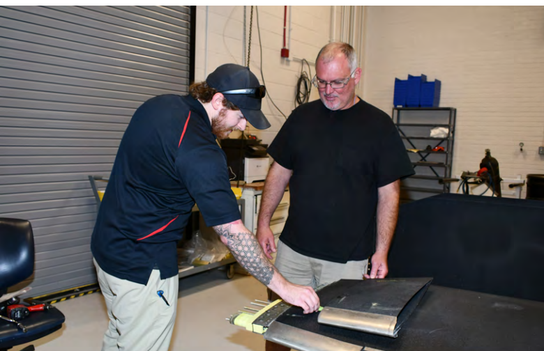
Joshua Peedin, left, senior rotor systems engineer for the H-53 Fleet Support Team, and Robert Call, work leader for the dynamic components shop, inspect the weights used to balance an H-53E rotor blade. Fleet Readiness Center East uses the universal static balance fixture to balance rotor and tail blades for the H-53E, V-22 and H-1 helicopters, and the H-53K program plans to use the fixture to balance its blades as well.
