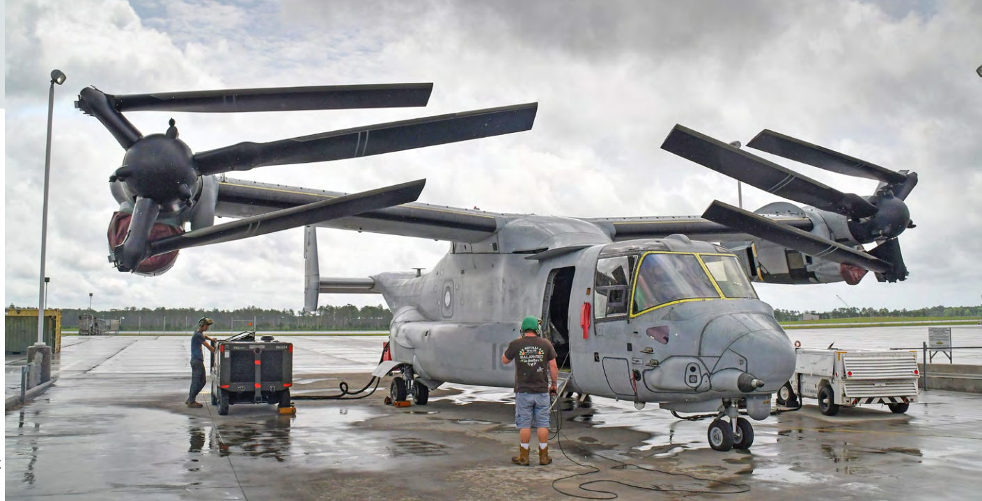
Fleet Readiness Center East (FRCE) artisans ready an MV-22 Osprey for “ground turn” which is an essential operational test of all of the aircraft’s systems and components. This is one of the last major steps that must be accomplished before this aircraft can be determined to be “Safe for Flight.”
