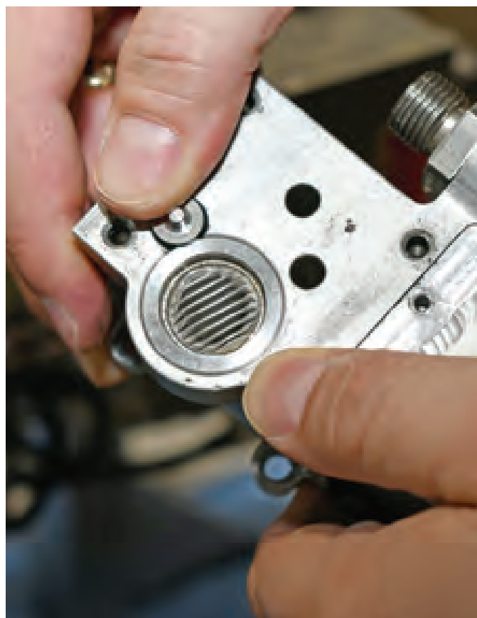
A close view of a clutch servo-valve filter on an auxiliary power unit for a V-22 Osprey. This quarter-sized filter is part of a critical oil line that helps engage the APU clutch to the midwing gearbox in order to start the V-22's main engines.
