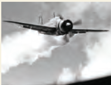
The Judy came in two versions that used two different power plants. While the D4Y3, shown in the cover illustration, used a Japanese designed air-cooled radial engine, the earlier D4Y2 used a liquid-cooled vee engine as shown here. As with many aircraft with such an engine, the aircraft's design required a long nose which often restricted the pilot's view forward, hence the standing observer helps the pilot taxi.
