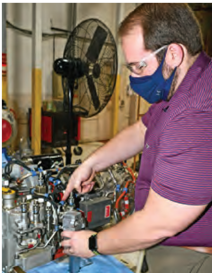
Rob Wansker, FRCE V-22 Power and Propulsion Auxiliary Power Unit (APU) senior engineer, indicates the location of the clutch servo-valve filter on a V-22 Osprey APU. Wansker's team developed a process to clean these filters after a supply backlog made the critical filters briefly unavailable to Navy and Marine Corps maintainers.
