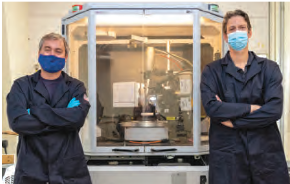
Dr. Randall McClain, left, and Dr. Ben Harvey stand in front of a single crystal X-ray diffractometer, which is used to determine the chemical structure of molecules.
