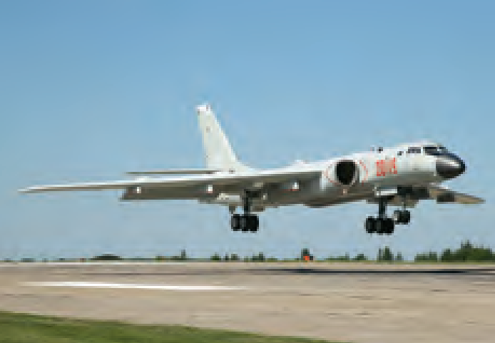
The Kilo model of the long-lived Badger is both a bomber as well as a missile-strike aircraft, and is powered by two non-afterburning turbofans.
