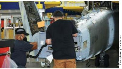
Aircraft mechanic Mario Orejudos (left) and aircraft mechanic apprentice Obeiean Pagaduan (right) install tail pylon swivel fittings on an MH-60 aircraft.
