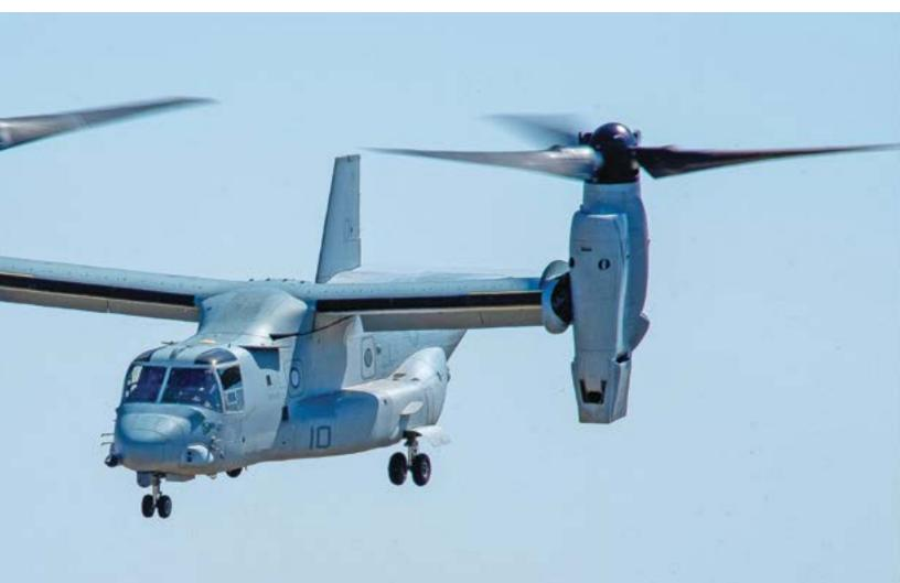
HX-21's MV-22 Osprey departs NAS Patuxent River during its first functional flight test with the modified nacelles and wiring.
