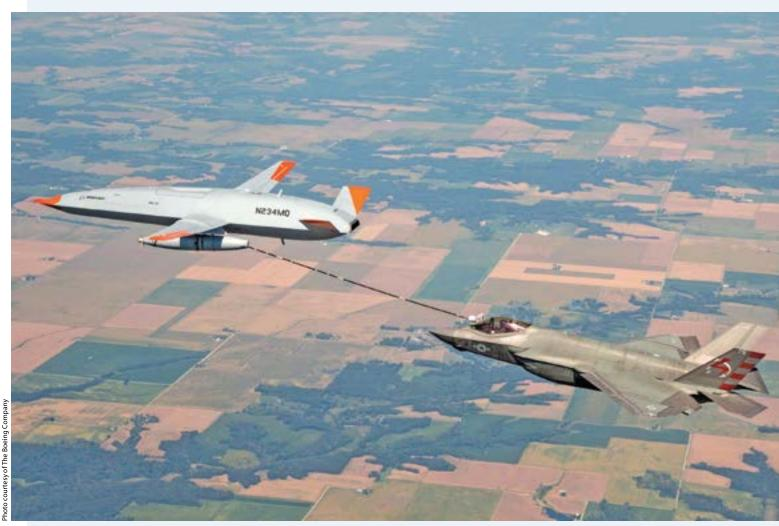
MQ-25 test asset, known as T1, conducts its first aerial refueling test flight with an F-35C Lightning II Sept. 13 near MidAmerica St. Louis Airport in Mascoutah, III.
