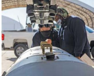
From left to right, Aviation Ordnanceman (AO) Airman Raul Ramos, AO 2nd Class Kailey Neugebauer and AO 1st Class Tyler Jacobson connect the NGJ-MB pod to the support equipment cables that will detach it from the EA-18G Growler wing during a logistics demonstration held at Naval Air Station Patuxent River, Md.
