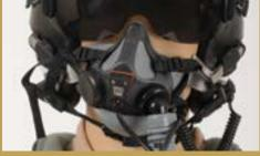
Visor profile does not match oxygen mask profile. Oxygen mask is not aligned properly on face.
