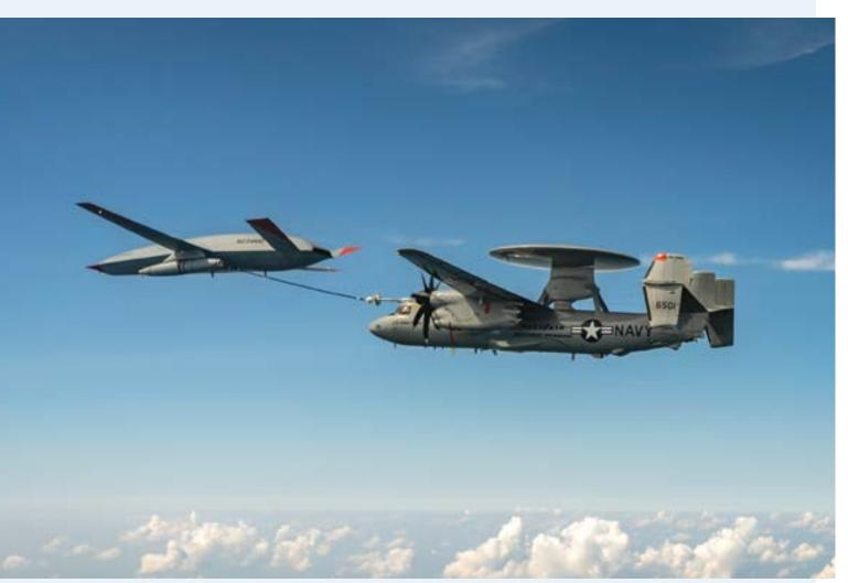
The MQ-25 Stingray test asset conducts its first aerial refueling flight with an E-2D Advanced Hawkeye Aug. 18 at MidAmerica Airport in Illinois.
