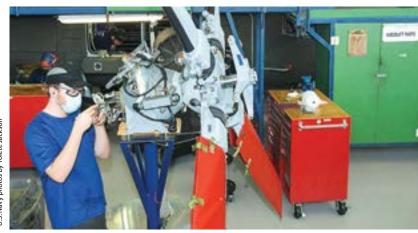
Clay Johnson, an aircraft mechanic apprentice with Fleet Readiness Center Southeast's vertical lift production line, performs maintenance on an H-60 tail rotor gear box.
