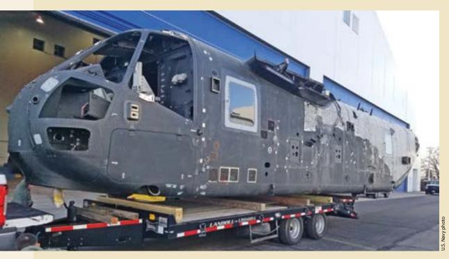
The former CH-53K King Stallion structural test aircraft arrived in Maryland in March and will be restored before being used for cargo certification and qualification.
