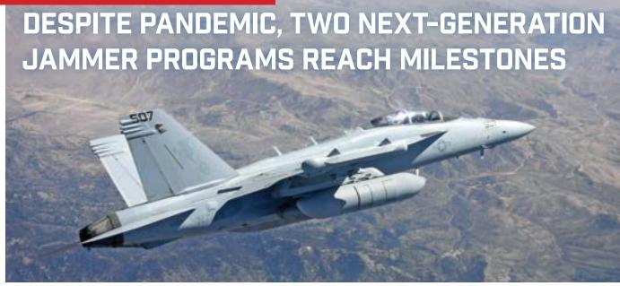
Air Test and Evaluation Squadron (VX) 31, located in China Lake, Calif., conducts a flight test with Next-Generation Jammer Mid-Band (NGJ-MB) and its host aircraft, EA-18G Growler.
