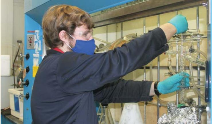
Chris Walkling, a chemical engineer working in the NAWCWD research department, conducts a distillation of a biosynthetic fuel component. "The benefits to the warfighter are clear. If we can provide them with biosynthetic fuels that outperform those derived from petroleum and can be produced domestically or in the field on-demand, we are giving them an advantage over their adversaries."
