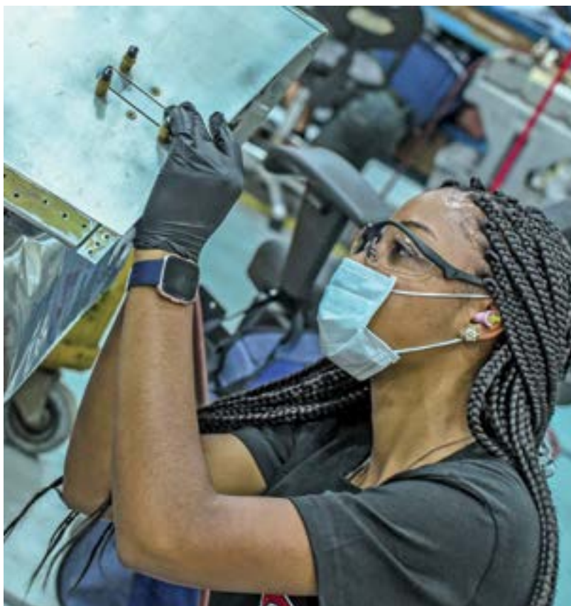
Fleet Readiness Center Southeast's sheet metal apprentice Jayda Hall installs forward latches for a P-3 Orion door in the Small Surface Shop.
