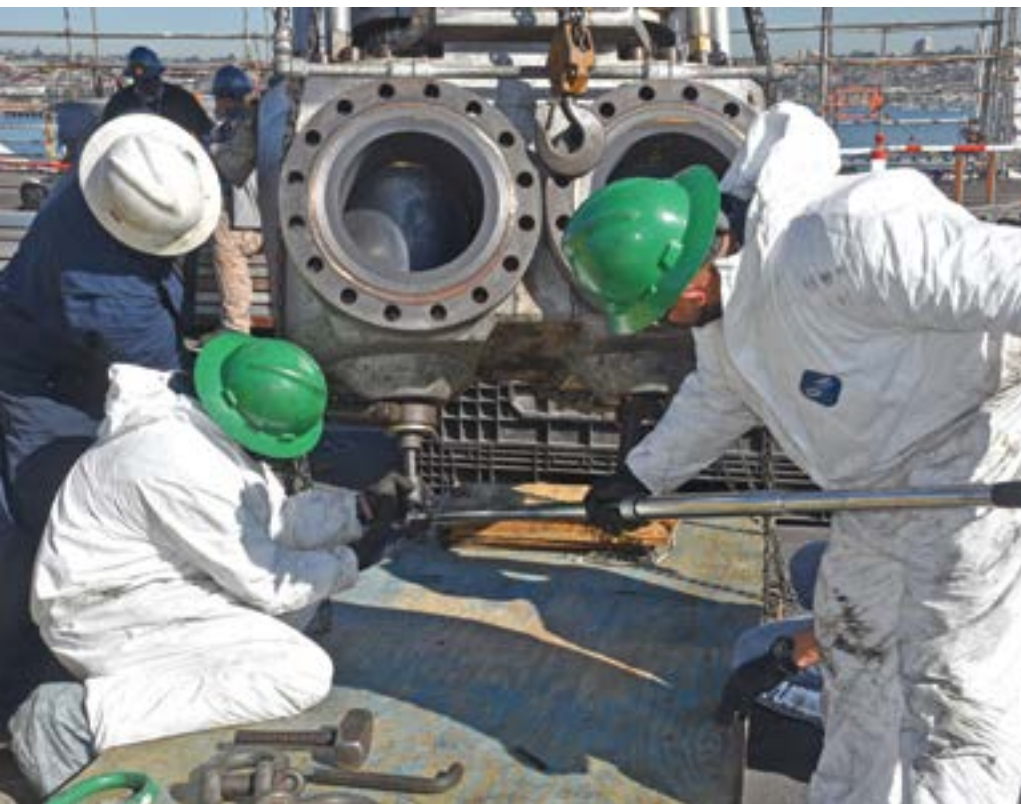
Onboard USS Abraham Lincoln (CVN 72), Fleet Readiness Center Southwest Voyage Repair Team artisans remove the catapult launch valve as part of the maintenance program to the ship's catapult system.
