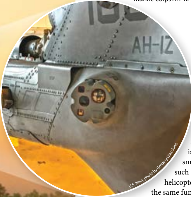
Marines with Aviation Combat Element, Marine Rotational Force-Darwin conduct a practice landing with an AH-1Z Viper at RAAF Base Darwin, Australia. The photo inset depicts a Distributed Aperture Infrared Countermeasure sensor tail-mounted on a Marine Corps AH-1Z aircraft.
