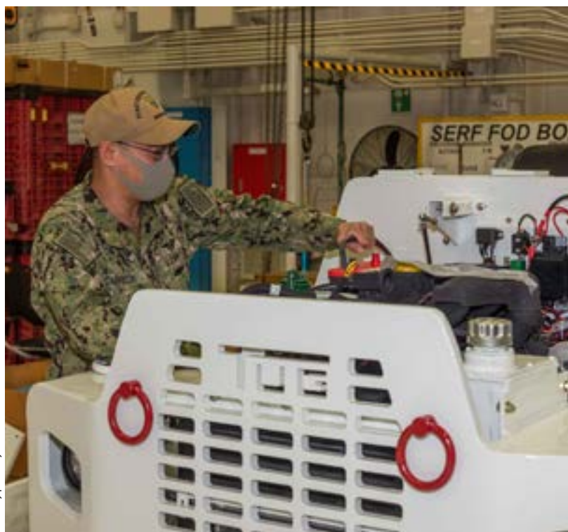
Aviation Support Equipment Technician Chief Petty Officer Palmer Carreon, with Fleet Readiness Center Western Pacific, performs a visual inspection on the engine of a shore tow tractor being serviced aboard Naval Air Facility Atsugi, Japan.
