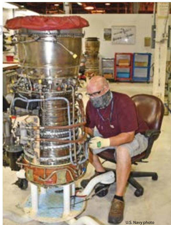
Mike DeLuzio, an aircraft engine mechanic in the T64 engine shop at Fleet Readiness Center East, installs the electrical harness to the overspeed switch on a T64 engine.
