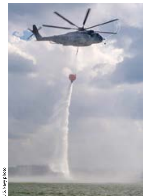
An MH-53E Sea Dragon, assigned to Helicopter Mine Countermeasure Squadron (HM) 12, conducts aerial firefighting capability testing with a Bambi Bucket.
