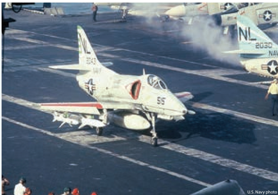
In 1967, an Iron Hand VA-155 A-4E taxis up the flight deck of the USS Coral Sea (CVA 43) armed with AGM-45A Shrikes and AGM-12A/B Bullpups on the outboard and inboard pylons, respectively.
