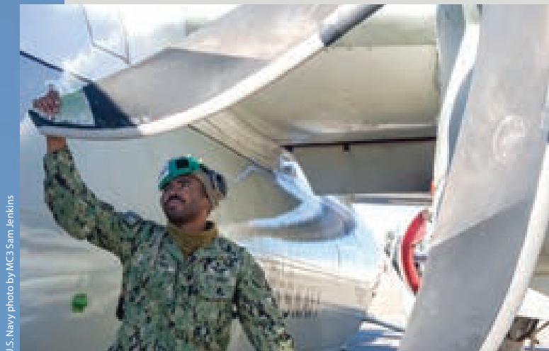
Aviation Machinist Mate (AD) 1st Class Terrell Williams, with VRC-40, inspects the propellers for damage on a C-2 on the flight line onboard Naval Station Norfolk, Va.
