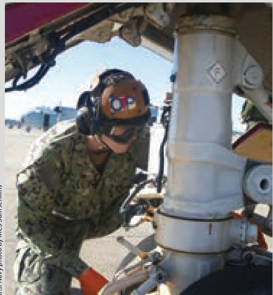
Aviation Electronics Technician (AT) Airman James Stith, with VRC-40, lubricates the landing gear on a C-2A.
