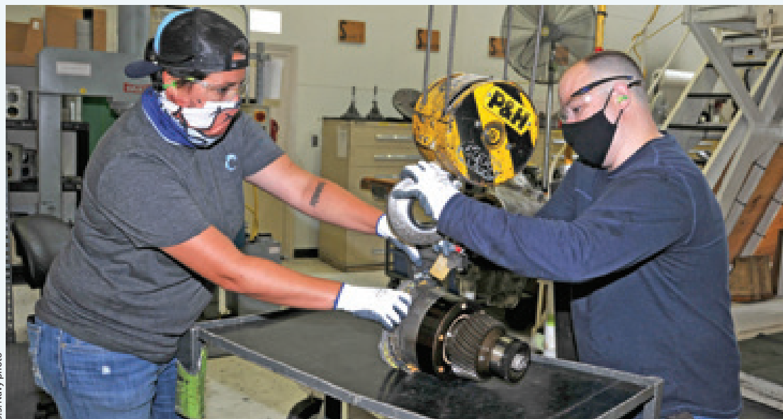
Crystal Gent, left, a Fleet Readiness Center East aircraft mechanical parts repairer apprentice, assists Joshua Maragni, aircraft mechanical parts repairer, in using a crane to lift a nose gearbox assembly for the H-53 helicopter.
