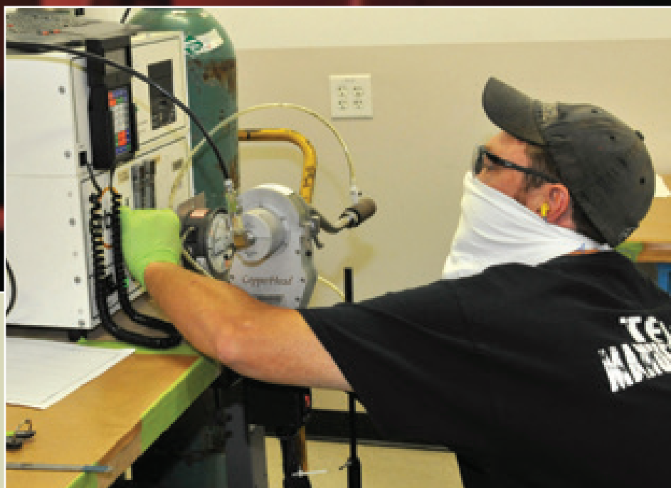
Robert Warmack, Fleet Readiness Center East welder, sets up an Orbital Welding Machine to weld fittings onto a titanium fuel line tube for the V-22 Osprey. FRCE is the only DOD aircraft maintenance facility with the capability to weld titanium hydraulic and fuel line tubes for the V-22 aircraft.
