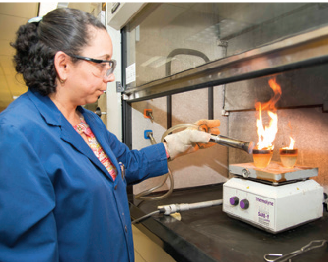
A fuels and lubricants chemist at NAWCAD conducts jet and diesel fuel quality tests in a propulsion and power lab at NAS Patuxent River.
