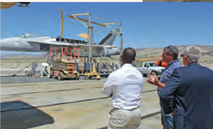
An F-14 MANPADS (man-portable air defense system) is tested in static condition, tower mounted at the WSL.
