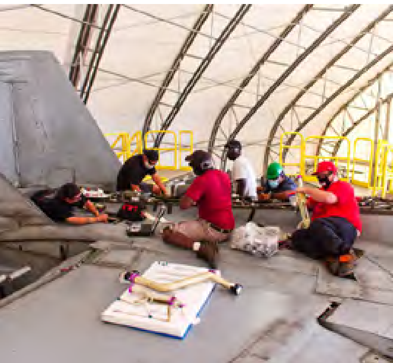
NAMCE maintainers rebuild long-term down F/A-18 Super Hornets inside the 73,800-square foot tension fabric structure at NAS Lemoore.
