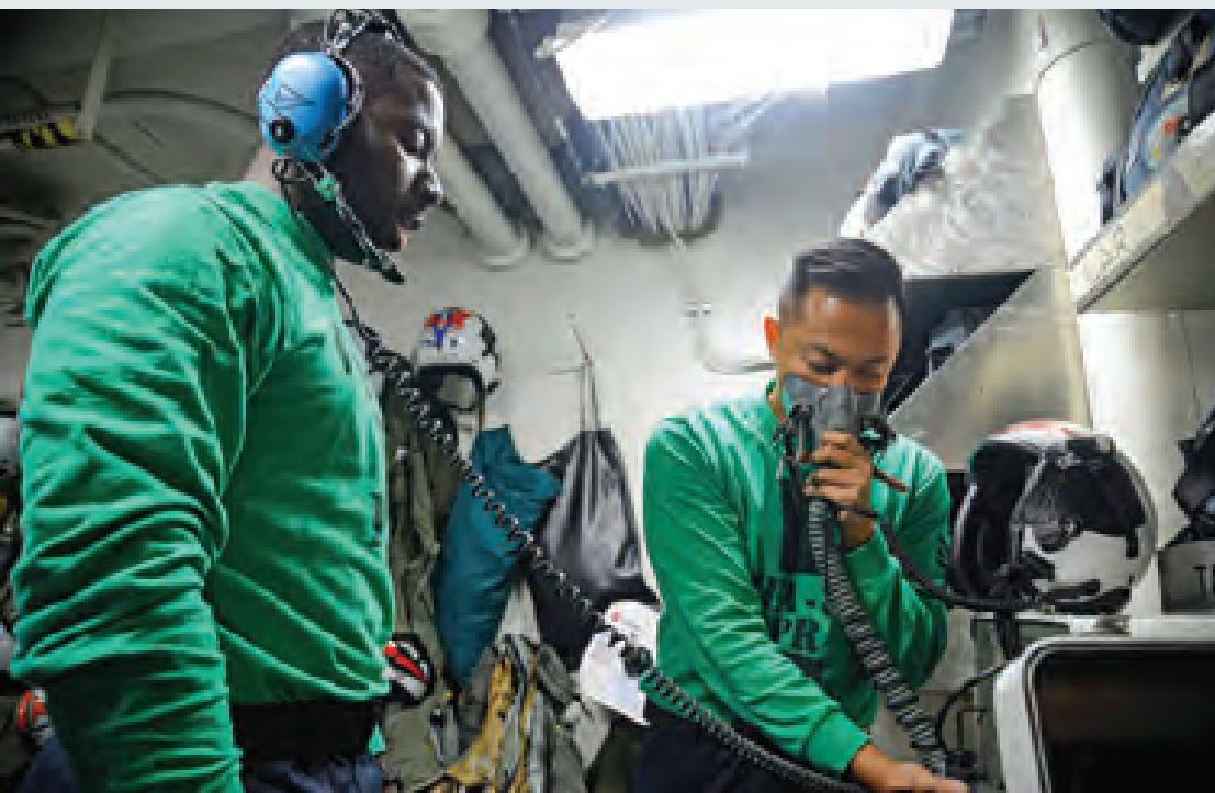
Aircrew Survival Equipmentman Airmen, assigned to the "Sunliners" of Strike Fighter Squadron (VFA) 81, test oxygen flow in pilot gear in a paraloft aboard aircraft carrier USS Harry S. Truman (CVN 75).
