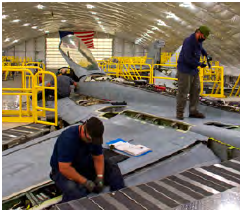
NAMCE maintainers rebuild long-term down F/A-18 Super Hornets inside the 73,800-square foot tension fabric structure at NAS Lemoore.
