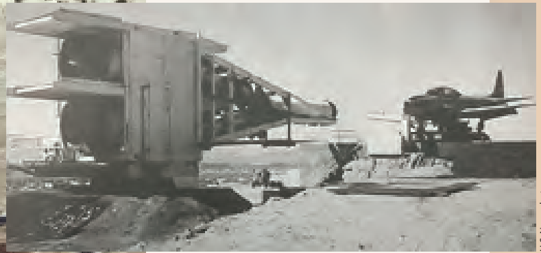
A T-33B aircraft is set up for a test at the WSL's original two-engine High Velocity Airflow System (HIVAS) circa 1975.
