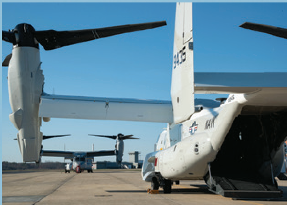
The CMV-22B is capable of internally transporting the F-35C Lightning II engine power module via its cargo bay.
