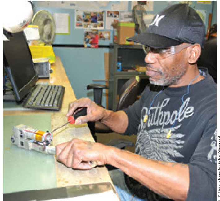
Richard P. Boyd, an electrical equipment repairer at Fleet Readiness Center East (FRCE), works on the motor for an H-53 tail skid actuator.
