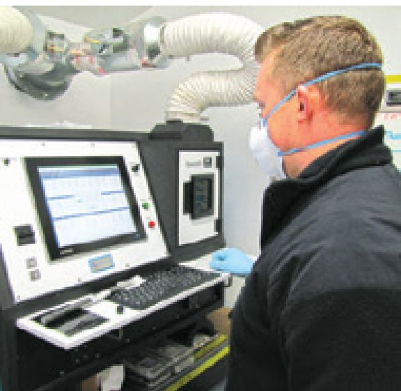
AD2 Adam Sack, left, performs oil analysis checks on the spectrometer. Center, Aviation Machinist's Mate Airman, (ADAN) Juvonni Headd disassembles a LAU-17F/A for inspection at FRCW DET Fallon. AT2 Zachary Smith, right, performs calibration checks on a De-Ice Test set.
