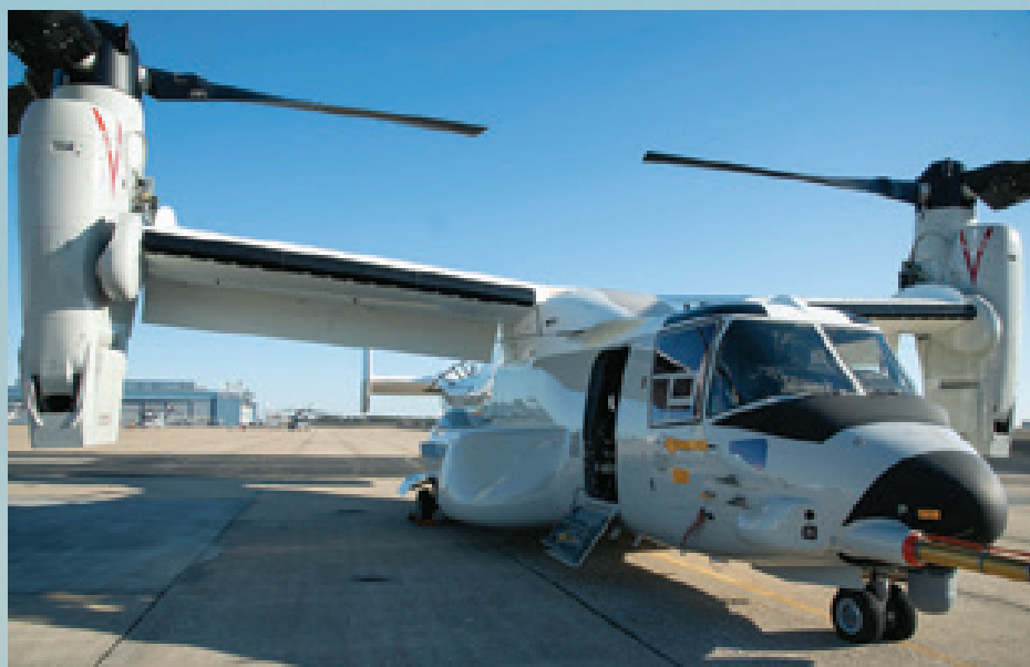
This angle highlights one of the new expanded sponson tanks on the CMV-22B on the flight line at Naval Air Station Patuxent River, Md.
