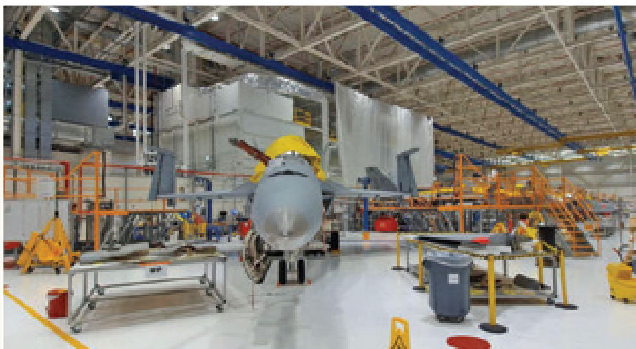
An F/A-18 Super Hornet undergoes Service Life Modification at The Boeing Company's St. Louis facility in late 2019.
