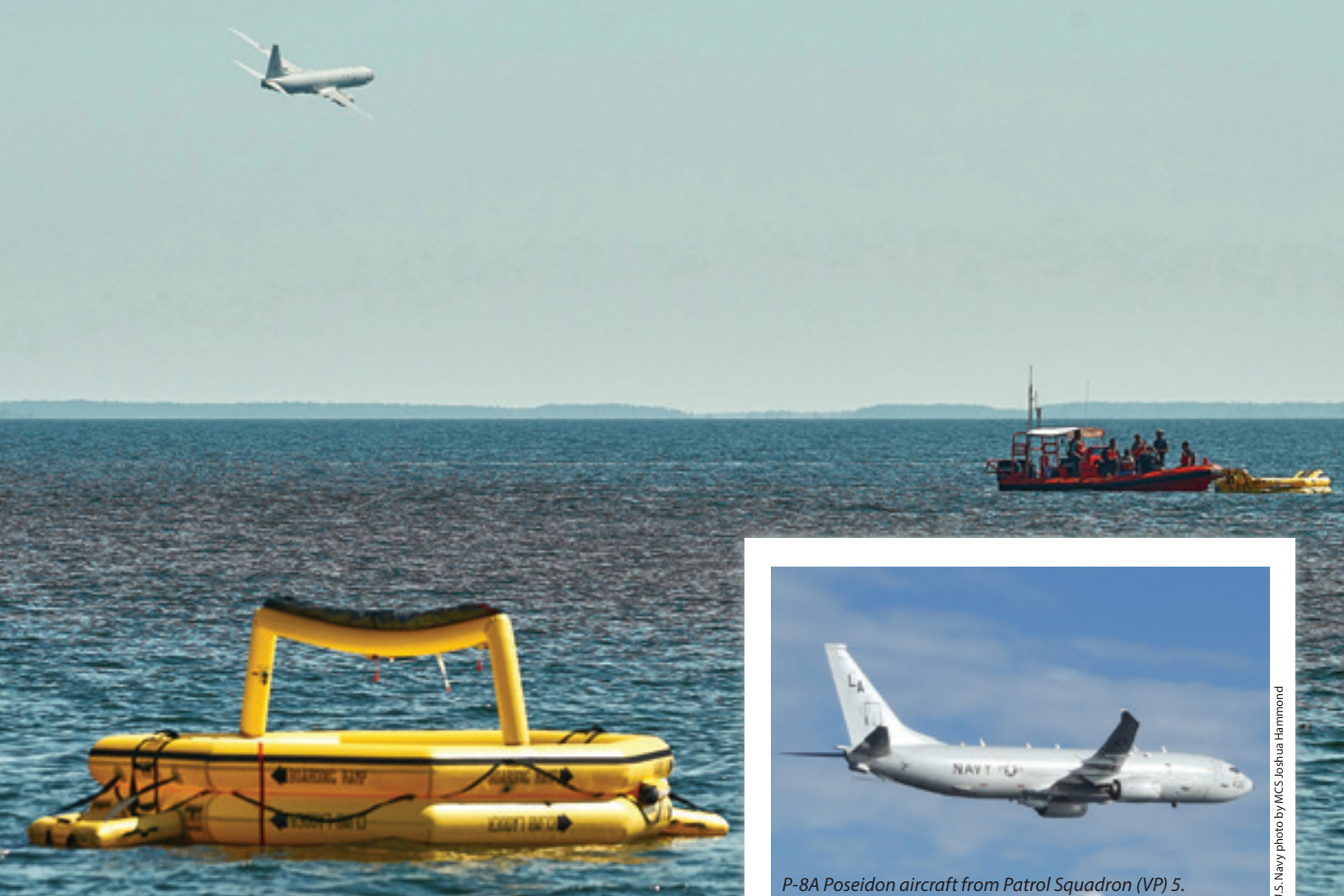
During a test, a P-8A Poseidon drops the advanced search and rescue kit, the UNIPAC III, approximately 5 miles off the coast of the Naval Air Station Patuxent River.
