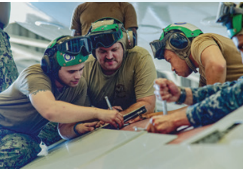
Aviation Structural Mechanic 1st Class Mark Coufal, a Center for Naval Aviation Technical Training Unit Norfolk instructor, center, provides hands-on training in E-2 Hawkeye aircraft flap actuator removal to maintenance technicians assigned to the "Bear Aces" of Carrier Airborne Early Warning Squadron (VAW) 124.
