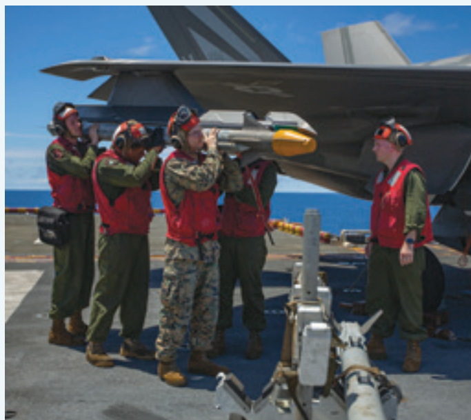
Ordnance Marines load an AIM-9X Sidewinder missile onto an F-35B Lightning II fighter aircraft.
