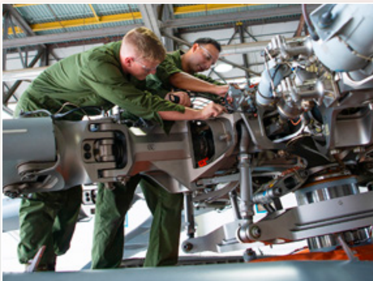
Pfc. Tanner Hawkins (left) and Cpl. Elijah Cervantes, Marine maintainers with VMX-1 inspect the rotor head of a CH-53K King Stallion from different angles during their first training rotation.
