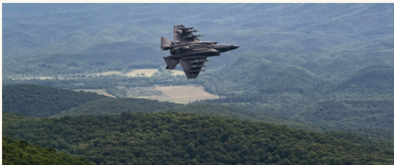
F-35 test pilot Dan Levin, Pax River Integrated Test Force, flies an Auto Ground Collision Avoidance System (Auto-GCAS) test flight in an F-35C Lightning II on a low level through West Virginia June 17. Flying the low level helps stress the Auto-GCAS software to confirm there are no false collision warnings while flying as close to the ground as operationally representative.
