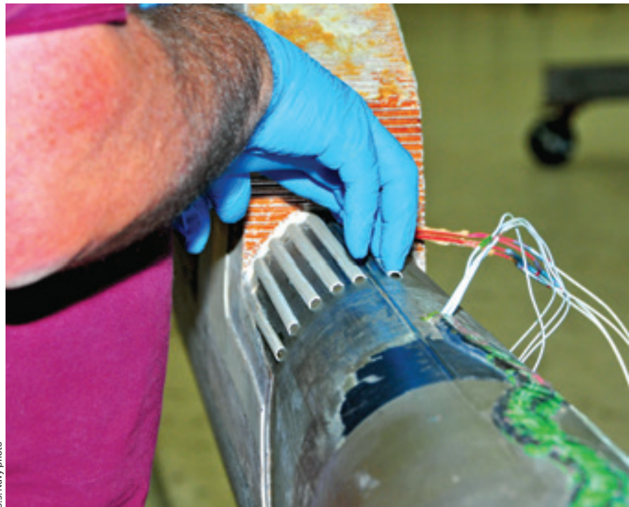
Bridgers keeps a firm press on an additively manufactured BIM vent to ensure it adheres to the spar of an H-53 blade.
