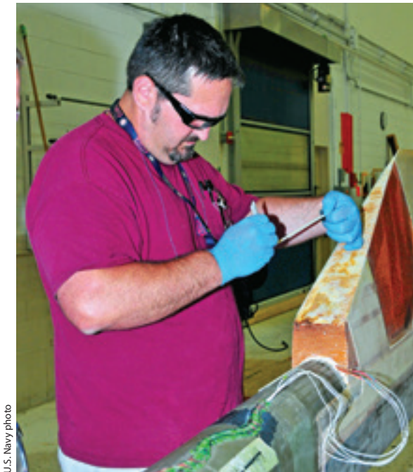
Todd Bridgers, an aircraft mechanical parts repairer applies a gel viscosity instant adhesive to a blade inspection method (BIM) vent—produced at Fleet Readiness Center East—before applying it to an H-53 blade.
