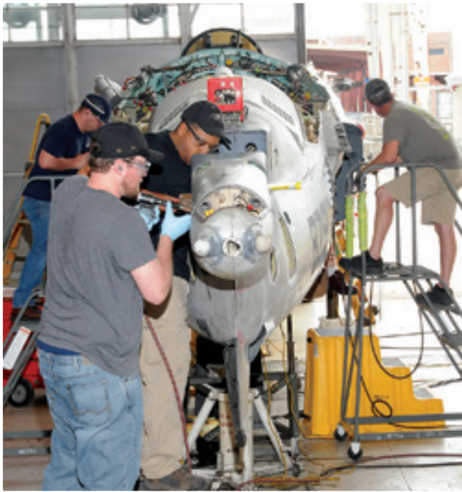
Artisans overhaul the fuselage of a Marine Corps Harrier on the FRCE AV-8 production line. In addition to the mandatory wear of bump caps, FRCE instituted a requirement for artisans to wear protective gloves. The two safety measures have greatly reduced head and hand injuries.
