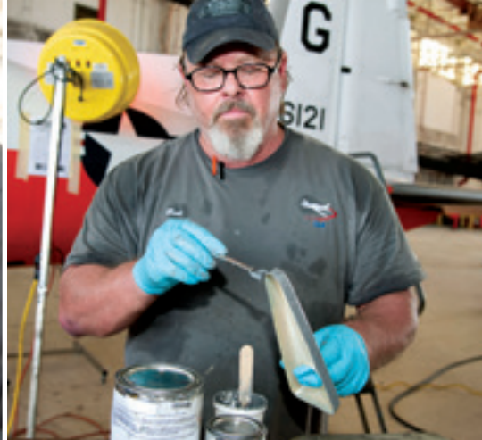
Thomas ensures the inner surface of the dorsal fin is clean and ready for rib installation. He then applies scrim cloth and adhesive to the new rib.
