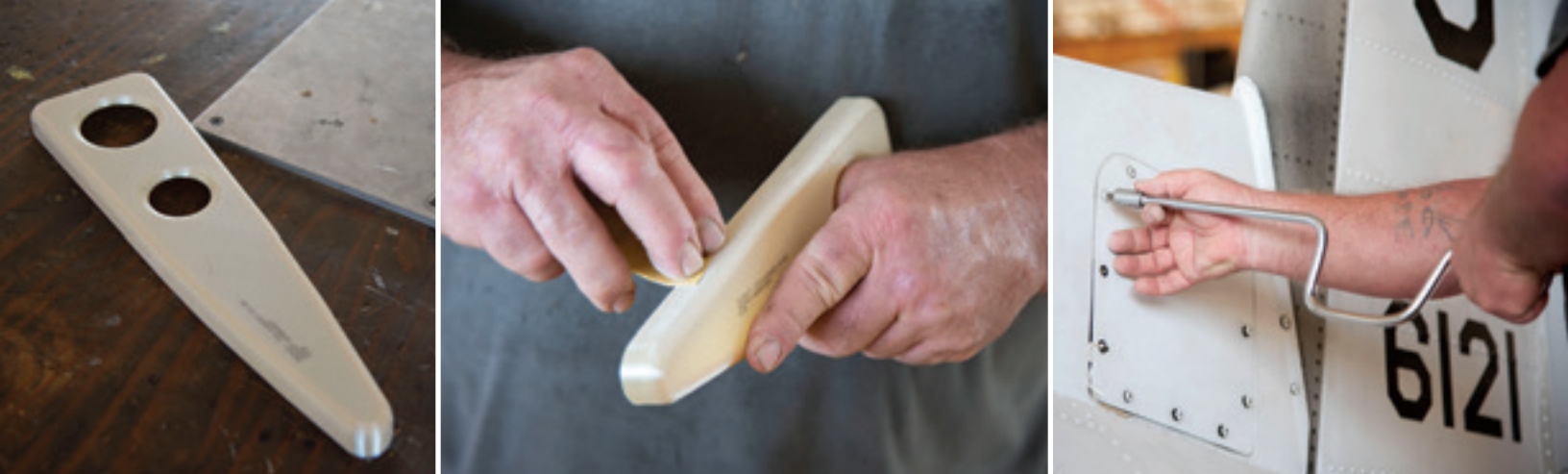
From left, a 3-D printed dorsal assembly rib awaits installation in a T-6B Texan. Robert Thomas, a conditional maintenance structural mechanic for Chief of Naval Air Training (CNATRA) at NAS Corpus Christi, Texas, scuff sands the rib prior to applying an adhesive. He then opens the dorsal fin access panel.
