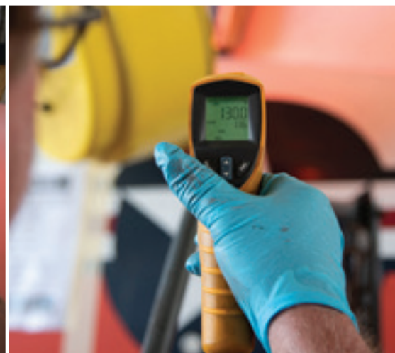
Thomas visually inspects his work to ensure proper bonding of the rib's faying surfaces. Heat lamps are placed on both sides of the aircraft to accelerate curing. Thomas uses a digital temperature laser gun to monitor the dorsal fin's skin temperature to ensure it doesn't exceed the recommended temperature.
