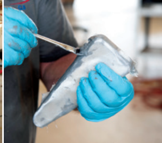
Thomas ensures the inner surface of the dorsal fin is clean and ready for rib installation. He then applies scrim cloth and adhesive to the new rib.
