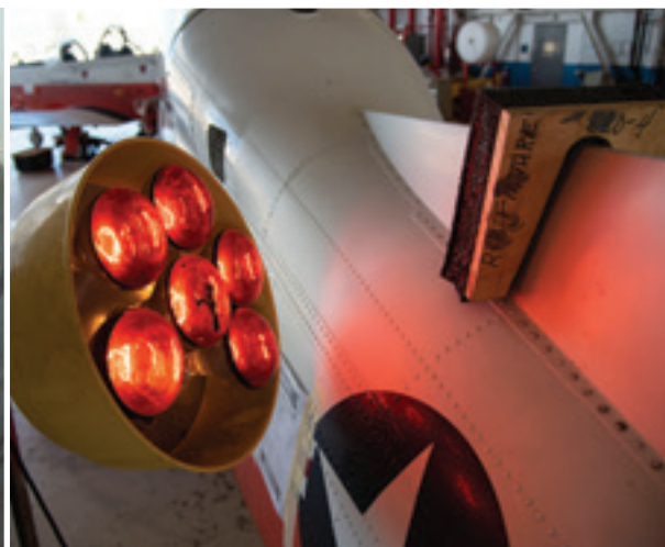
Thomas visually inspects his work to ensure proper bonding of the rib's faying surfaces. Heat lamps are placed on both sides of the aircraft to accelerate curing. Thomas uses a digital temperature laser gun to monitor the dorsal fin's skin temperature to ensure it doesn't exceed the recommended temperature.
