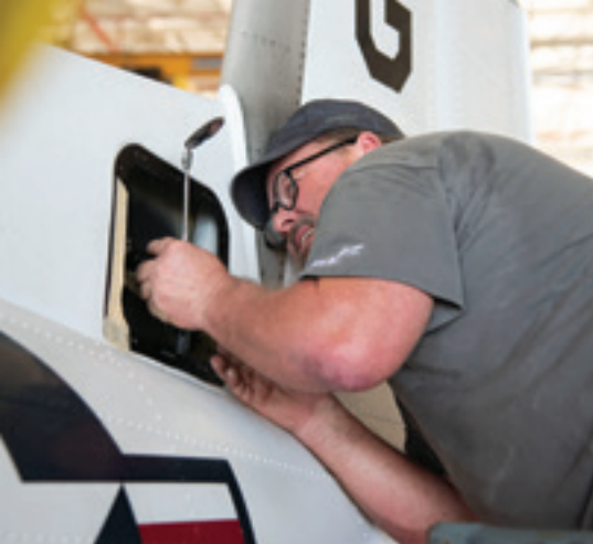
Thomas ensures the inner surface of the dorsal fin is clean and ready for rib installation. He then applies scrim cloth and adhesive to the new rib.
