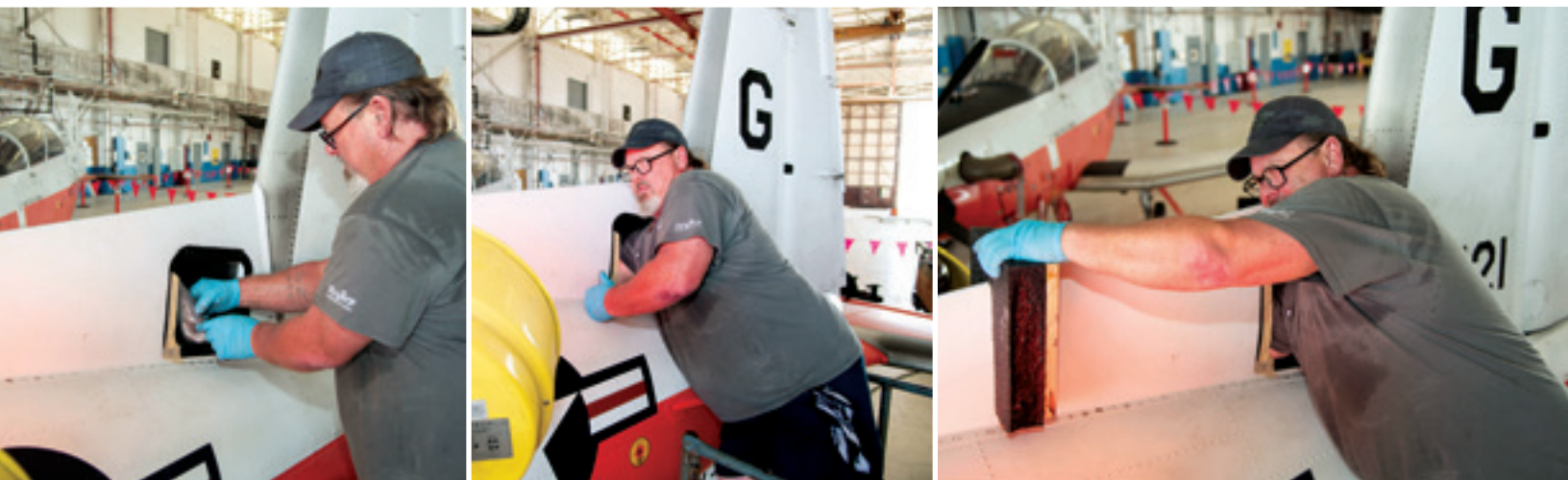
Thomas inserts the new rib through the access panel and positions the rib in place, then positions a fixture over the new rib to keep it in place while bonding occurs.
