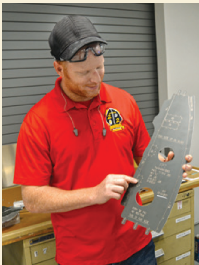
FRCSE sheet metal worker Josh Brown shows the etchings performed on the facility's new fiber laser cutter on a part template. What used to require two machines can now be done on a single laser cutter.
