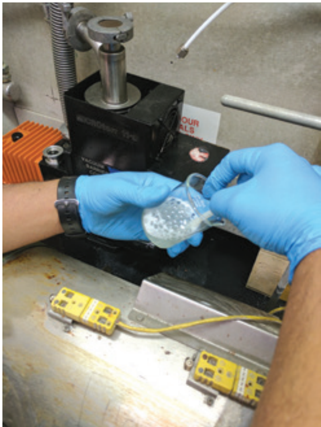
A close-up of gas flow verification using water as part of the process to grow the CNTs.
