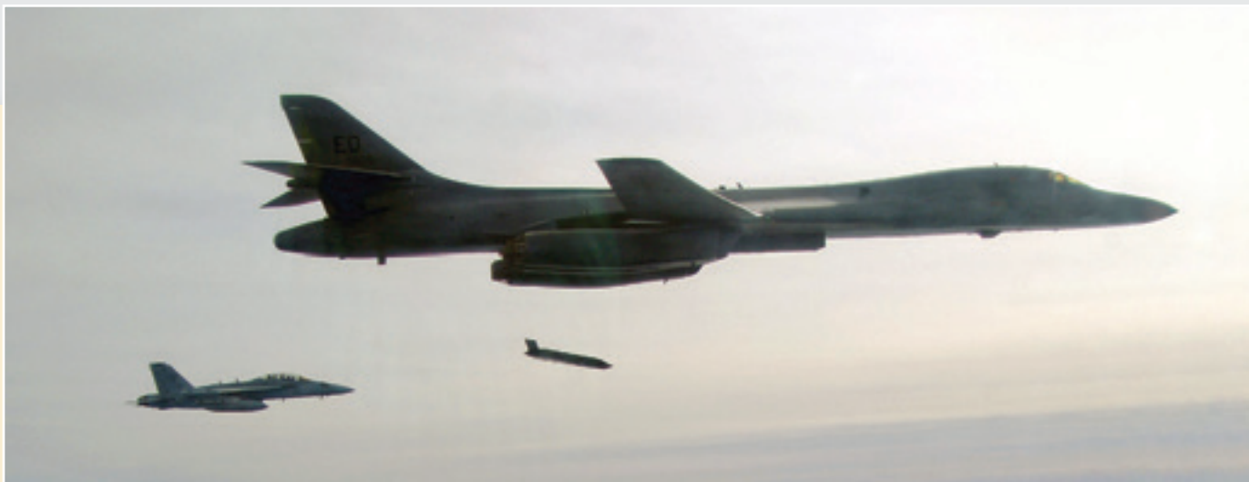
A U.S. Air Force B-1B Lancer releases the Navy's Long Range Anti-Ship Missile (LRASM) during a test event off the coast of California.
