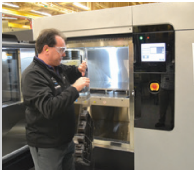
FRCSE tool designer Randy Meeker removes a part he printed on the plant's new Fortus 900 3-D printer Feb. 13.
