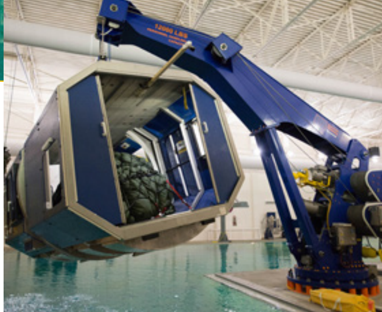
Known as the “dunk tank” or “dunker,” the METS was dropped several times into the pool as part of the demonstration. Each dunk was performed with the interior cargo arranged in a different configuration.
