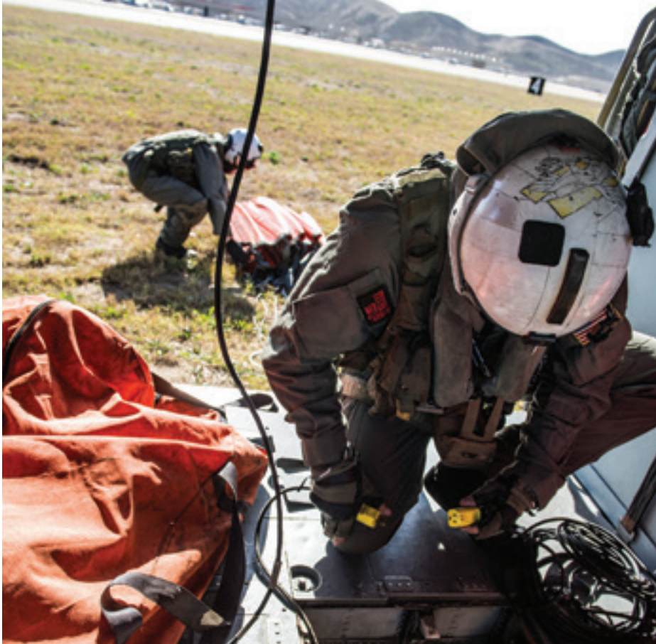
A naval aircrewman (Helicopter), assigned to the "Merlins" of Helicopter Sea Combat Squadron (HSC) 3, connects a "Bambi Bucket" to an MH-60S Seahawk helicopter in support of aerial firefighting efforts.
