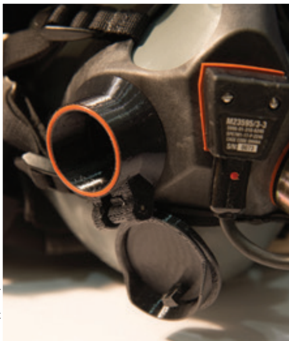
A 3-D printed flip-top valve as applied to a T-45 Goshawk breathing mask. The valve was created to allow T-45 students to continue syllabus flights while fixes were made to the aircraft’s Onboard Oxygen Generation System.
