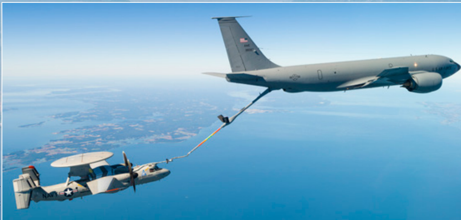
The aerial refueling-equipped E-2D engages the refueling drogue trailing from a U.S. Air Force KC-135 Stratotanker.
