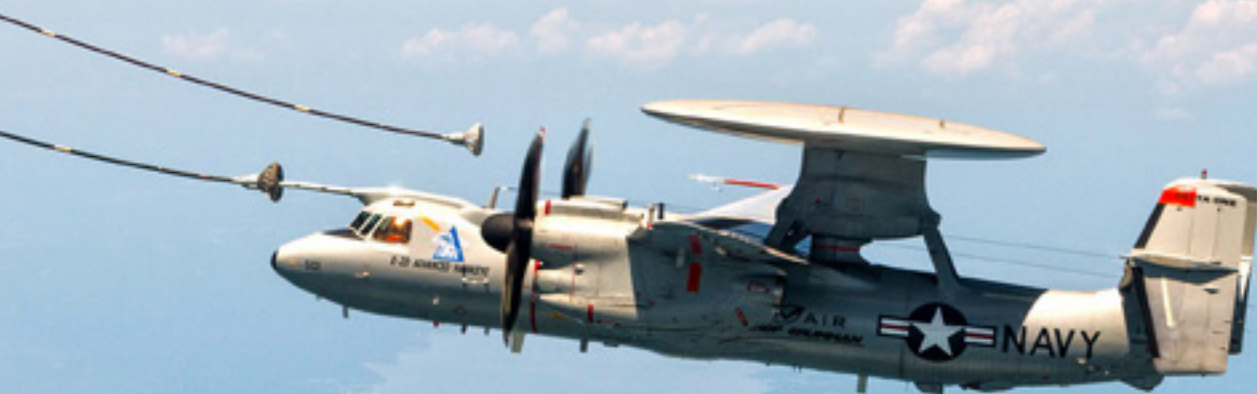
The aerial refueling-equipped E-2D Advanced Hawkeye receives 162 pounds of fuel from a U.S. Navy KC-130 Hercules during its first in-flight fuel transfer test July 14.
