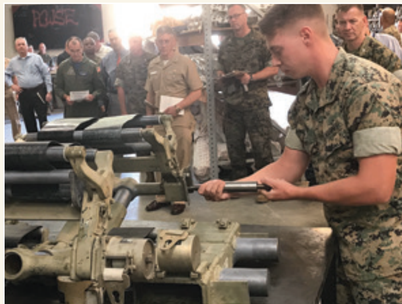
Marine Lance Cpl. Richard Happ demonstrates the redesigned AERO-74 slide hammer that allows users to remove a threaded attachment in order to avoid excessive maintenance delays. MALS-13 hopes to share this innovative idea with all type/model/series that use the AERO-74.
