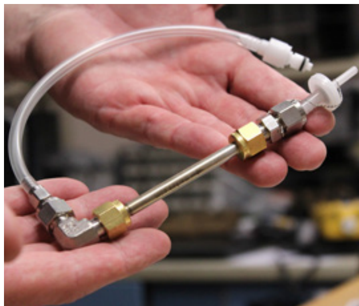
The above sorbent tube is a reusable metal tube that attaches to the aircrew's oxygen breathing regulator and is used to sample the oxygen flow for potential contaminants. These samples allow engineers to monitor and assess the quality of the breathing gas that was delivered to aircrew during flight.
