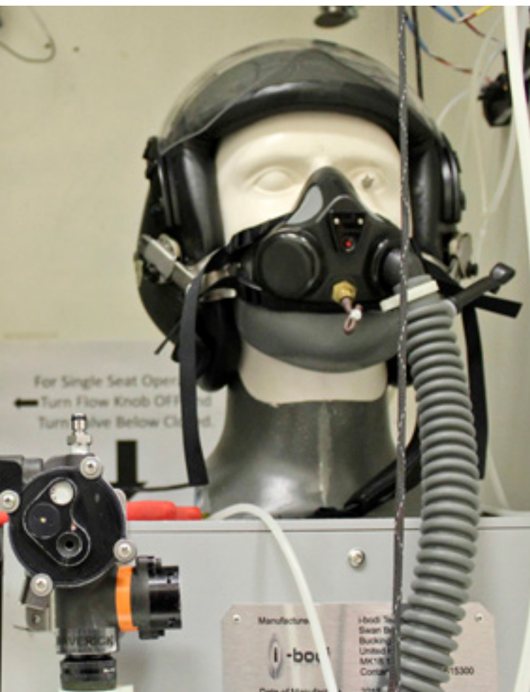
The Naval Air Warfare Center Aircraft Division Altitude Lab uses these mechanical breathing machines to simulate aircrew breathing while testing oxygen systems, such as the On-board Oxygen Generation Systems (OBOGS).
