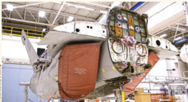
Boeing will examine the two Super Hornets' forward fuselages and wings, while Northrup Grumman will inspect the center aft fuselages (pictured above).
