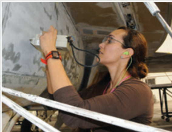
Jennifer Nunez, a materials engineer with FRCSE, uses a surface coding tester to detect the presence of conductive coating on an F/A-18E/F Super Hornet during the stripping process.
