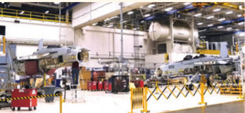
In preparation for the first four F/A-18E-F Super Hornets set to enter the Service Life Modification (SLM) program in 2018, Boeing recently despoiled—or split in half—two retired, high-use jets to examine them for fatigue and validate required maintenance.
