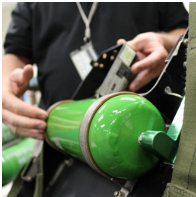
The emergency oxygen cylinder is located in the ejection seat. It holds about 200 liters of high pressure gaseous oxygen used during an ejection and as an emergency backup to the OBOGS.
