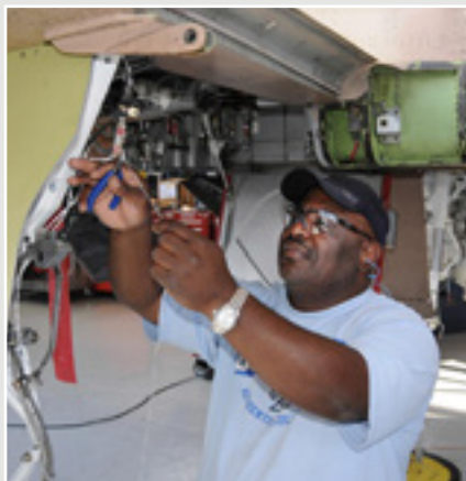
Artisan Robert Newberry installs a landing gear harness at Fleet Readiness Center Southeast (FRCSE).
