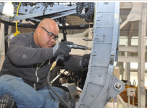
Sheet metal mechanic Kris Dipraseuth repairs a structural crack on an H-60 Seahawk at Fleet Readiness Center Southwest (FRCSW).
