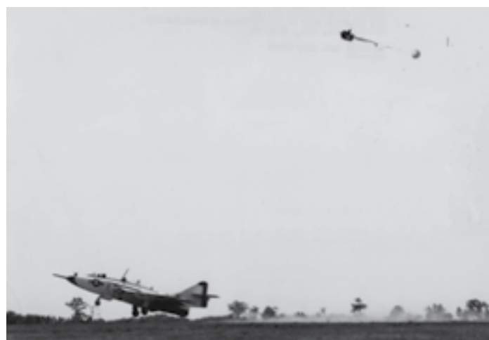
The ground-level ejection seat is demonstrated at the Naval Air Test Center at NAS Patuxent River, Md., 28 August 1956. A successful ejection was made by Lt. Sydney Hughes, British Royal Air Force, from an F9F-8T Cougar flying just above the ground at 120 mph.
