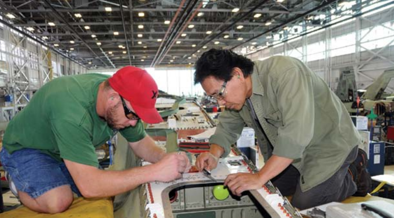
Lonnie Conditt, left, and Narom Orr, right, both machinists at Fleet Readiness Center Southeast in Jacksonville, Fla., measure holes to ensure alignment of an F/A-18 Hornet part on the production line. (U.S. Navy photo by Victor Pitts)
