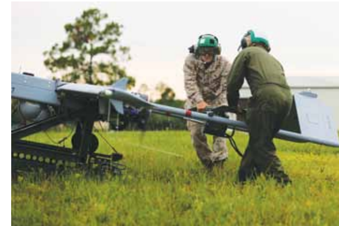
Lance Cpl. John M. Johnson Jr., left, and Lance Cpl. Jaleel Porter start the engine of a RQ-7B Shadow unmanned aerial vehicle during night flight training at Avon Park Air Force Range, Fla., 4 August. (USMC photo)
