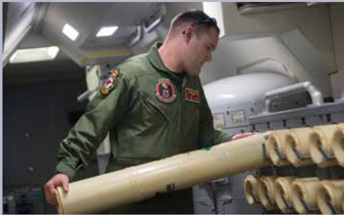
AWO2 Karl Shinn, assigned to the VP-16 War Eagles, unloads a sonobuoy from the rack aboard a P-8A Poseidon to prepare it for use during the early April search of the missing Malaysia Airline Flight MH370. (Photo by MCC Keith DeVinney)
